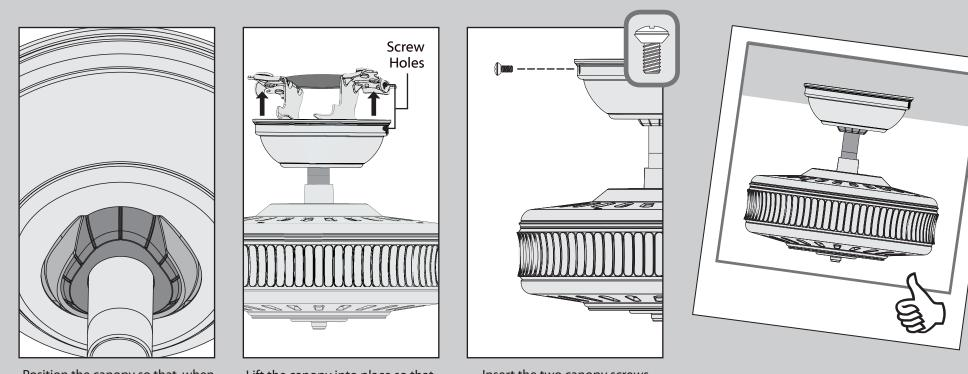
Position the canopy so that, when lifted into place, the canopy fits into the hanging bracket as shown.
